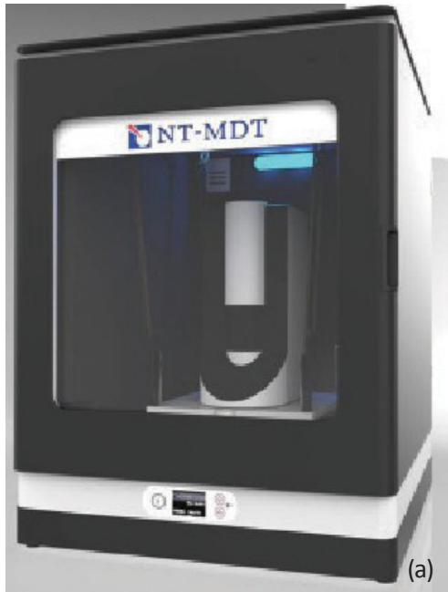
Fig 1 a-b. (a) A thermal cabinet. (b) Temporal graphs of the room and sample temperatures.
