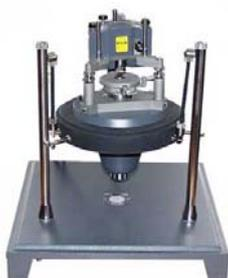
**Fig. 3** Passive vibroprotection system, SMENA head and automatic approach system (SOLVER P47H).
