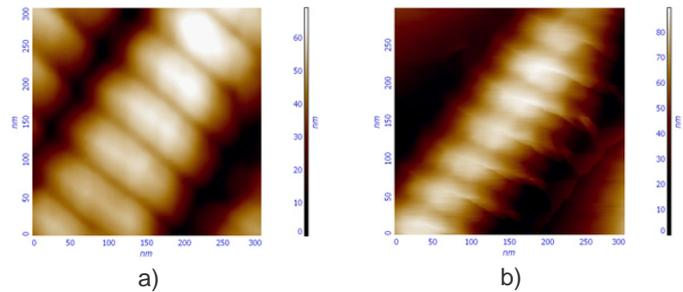
**Fig. 5** The topography of dry collagen fibril on glass obtained in semicontact mode: a) with noncontact Si probes NSG 11, aspect ratio 3:1.; b) noncontact Si "whisker" type probe NSC05 (NT-MDT), aspect ratio 10:1. It is obvious, that increase of probe aspect ratio leads to essentially increase of morphological features resolution.
