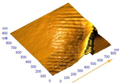
**Fig. 4** The collagen fibril in water on glass obtained in semicontact mode with contact Si probes CSG 11. The stripe periodicity of fibril and delicate structure of stripes are observed in surface profile.
