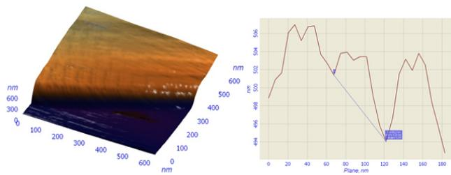
**Fig. 3** The collagen fibril in water on glass obtained in semicontact mode with contact Si probe CSG 11. The stripe periodicity of fibril and delicate structure of stripes were observed in surface profile.
