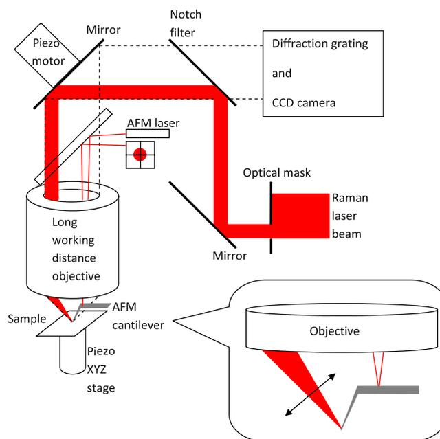
**Figure 1.** A schematic diagram showing the arrangement of the TERS system (NTEGRA Spectra) in an upright configuration. Note that the objective is used to focus laser light on the sample as well as to collect the scattered light at the spectrometer. The scattered light is shown with the dotted line boundaries.
