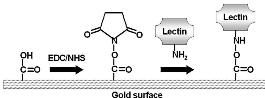
Fig. 1. Amine coupling procedure for immobilisation of lectins onto the thiolised golden surface.
