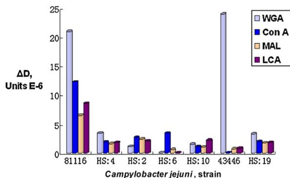
**Fig. 3.** Dissipation patterns from 5th overtone achieved from interaction between different *Campylobacter jejuni* strains and lectins. The analytical response was measured in the on-line mode 40 min after injection. Flow speed was set to  $50 \mu\text{L min}^{-1}$ . Ten mM PBS (containing 1 mM  $\text{Ca}^{2+}$  and 1 mM  $\text{Mg}^{2+}$ ) was used as a running buffer and 10 mM glycine-HCl (pH 2.5) was used as a regeneration solution.
