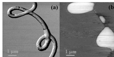
FIG. 1. AFM phase images of a single electrospun PEO fiber observed at (a) 23 °C and (b) 65 °C, showing the change from a solid cylindrical fiber to liquid droplets.
