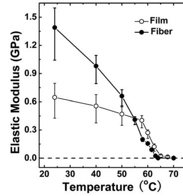
FIG. 3. Calculated elastic modulus of the PEO fiber and film from the experimental data fit of Eq. (1) as a function of temperature.
