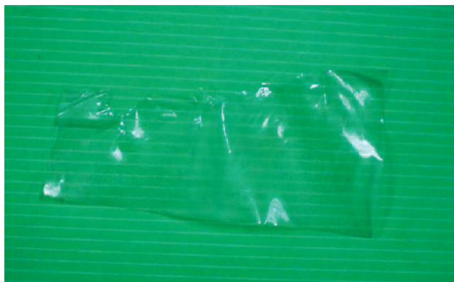
Figure 2. Photograph of [Bmim][BF 4 ]/polystyrene membrane produced from microemulsion polymerization of [Bmim][BF 4 ]/styrene/MAUM-Br (0.30/0.47/0.23), initiated by AIBN at 60 ^{\circ}\text{C} .
