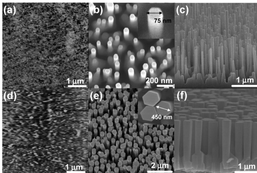
**Figure 5.** AFM images of sapphire substrates after etching in a 1 M NaOH solution (a) at room temperature for 15 s (height range 2 nm) and (d) at 150 °C for 10 min (height range 3 nm). (b, e) Top-view SEM images of NWs grown on parts a and d, respectively. The insets are magnified images and reveal hexagonal ZnO NWs and nanorods. (c, f) Side-view SEM images of parts b and e, respectively.
