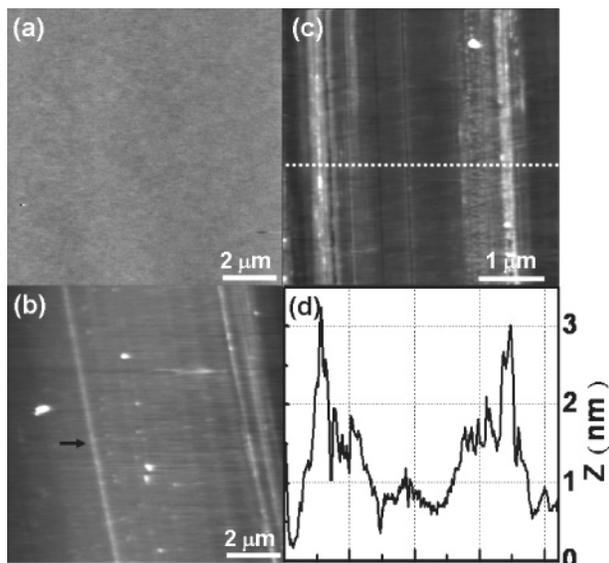
**Figure 1.** AFM images of (a) a bare sapphire surface (height range 1.8 nm) and (b) the surface (height range 6 nm) showing the presence of a long stripe region indicated by an arrow at a boundary after scratching. (c) Magnified view of the scratched area and (d) the corresponding cross-sectional profile along the dotted line in part c.
