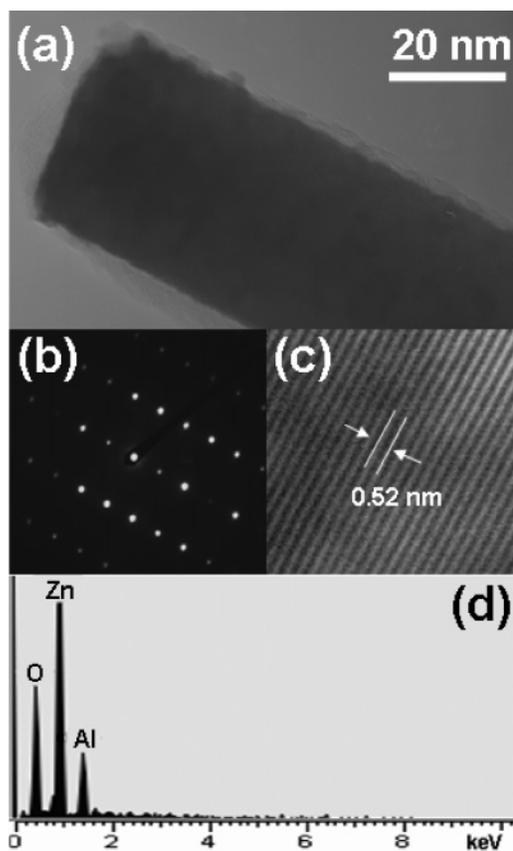
**Figure 3.** (a) TEM image of a ZnO NW with a diameter of 35 nm, (b) the corresponding selected area electron diffraction pattern, and (c) a high-resolution image exhibiting that the lattice constant  $c$  is 0.52 nm. (d) EDS spectrum of the ZnO NWs on sapphire.
