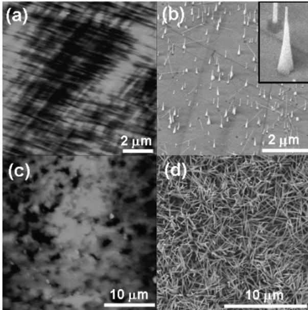
**Figure 4.** AFM images of sapphire substrates with rms roughness values of (a) 1.2 nm (height range 8 nm) and (c) 60 nm (height range 520 nm). (b, d) SEM images of the ZnO NWs in parts a and c, respectively. The inset is an enlarged view of one ZnO NW with a base diameter of around 150 nm.
