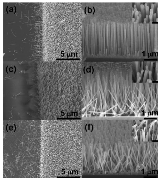
**Figure 2.** Top-view and side-view SEM images of NWs grown on scratched (a, b) sapphire, (c, d) glass, and (e, f) Si substrates, respectively. The scratched regions are on the right-hand side in the top-view images. The insets in parts b, d, and f are magnified images, and the scale bars are 200 nm long.
