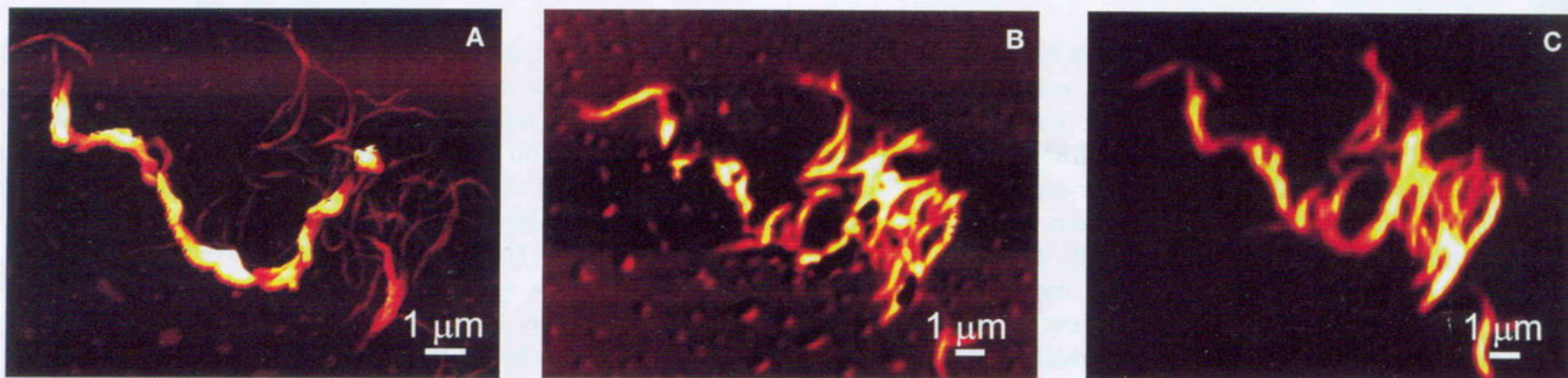
Fig. 2: SWNTs bundle: a) AFM image b) confocal optical image, c) confocal Raman image taken at \Delta\nu = 1587 \text{ cm}^{-1} .
