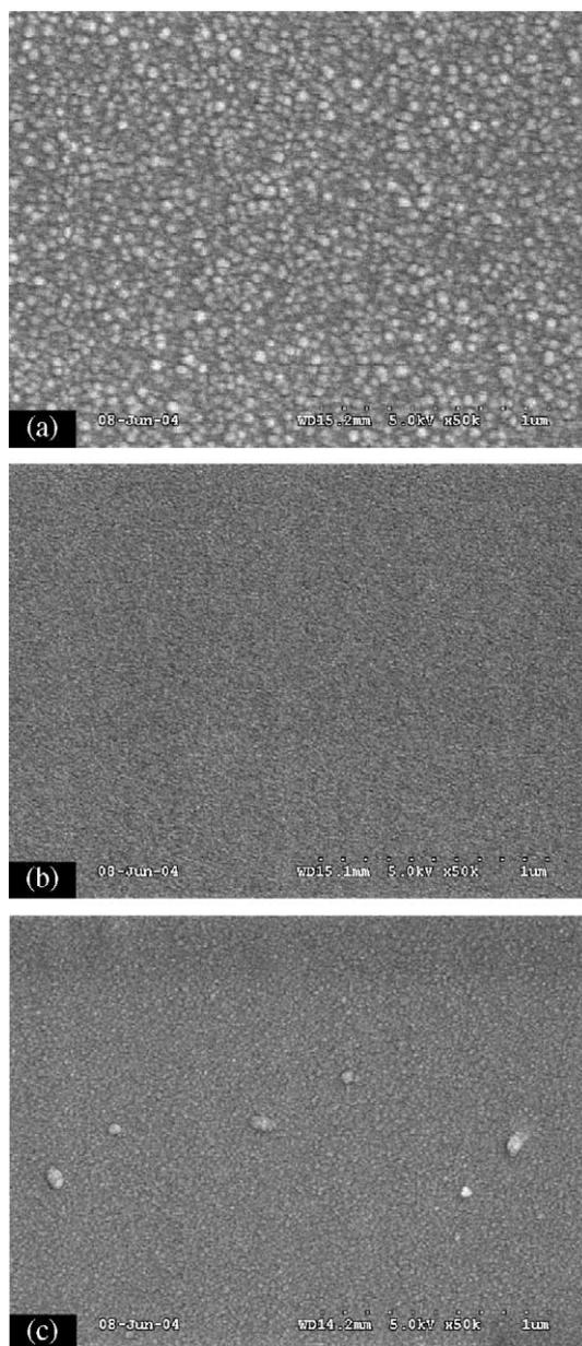
Fig. 2. The SEM micrographs of silicon films obtained under various  $W_2$  input (a) 15 W, (b) 30 W, and (c) 40 W.
