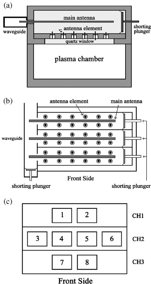
Fig. 1. The schematic drawings of (a) side view and (b) top view of the Triple-A microwave plasma source; and (c) the substrates positioning on holder.
