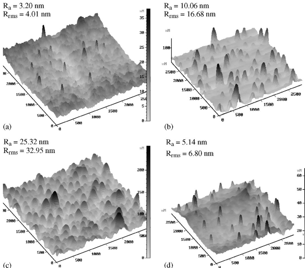
Fig. 3. The AFM topographies of silicon films obtained under  $F_{\text{H}_2}$  equal to (a) 10 sccm, (b) 20 sccm, (c) 25 sccm, and (d) 30 sccm.
