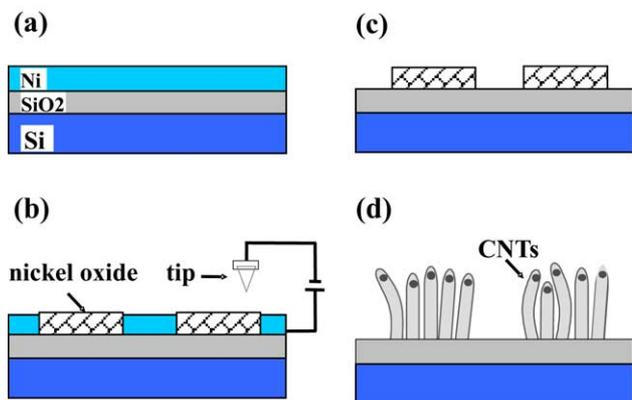
Fig. 1. A schematic process flow for the selective growth of CNTs on NiO<sub>x</sub> templates created by AFM: (a) the initial layered structure, (b) the AFM nano-oxidation, (c) the etching of nickel, and (d) the growth of CNTs.
