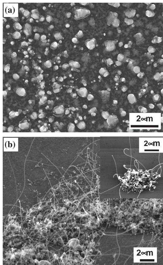
Fig. 3. SEM images of Ni films on not Ni-etched substrate after a 10-min nanotubes growth at (a) 700 °C and (b) 750 °C. The inset in (b) shows the SEM image of nanotubes grown on a NiO<sub>x</sub> square template of size 3 μm at 750 °C for 10 min.
