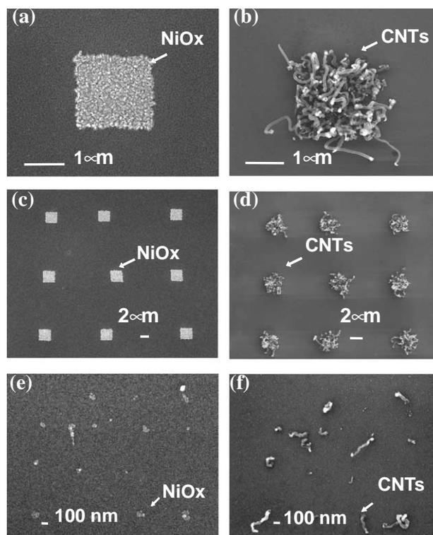
Fig. 2. SEM images of NiO<sub>x</sub> templates with varying geometries: (a) a single square of size 1.8  $\mu\text{m}$ , (c) a  $3 \times 3$  array of  $2 \mu\text{m} \times 2 \mu\text{m}$  squares, and (e) a  $4 \times 4$  array of dots of  $\sim 90$  nm in diameter. The corresponding CNTs grown on these NiO<sub>x</sub> templates at 700 °C for 10 min are shown in (b), (d), and (f), respectively.
