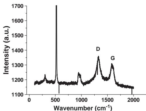
Fig. 4. Raman spectrum of nanotubes shown in Fig. 2(b) which were grown on a single NiO<sub>x</sub> square template of size 1.8 μm at 700 °C for 10 min.
