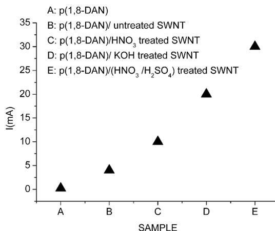
Fig. 8. Values of current intensity measured at 250 mV for series of films submitted to different treatments: (a) pure polymer film; (b) polymer film containing untreated nanotubes; (c) polymer film containing nanotubes treated by  $\text{HNO}_3$ ; (d) polymer film containing nanotubes treated by KOH; (e) polymer film containing nanotubes treated by the  $\text{HNO}_3/\text{H}_2\text{SO}_4$  mixture.
