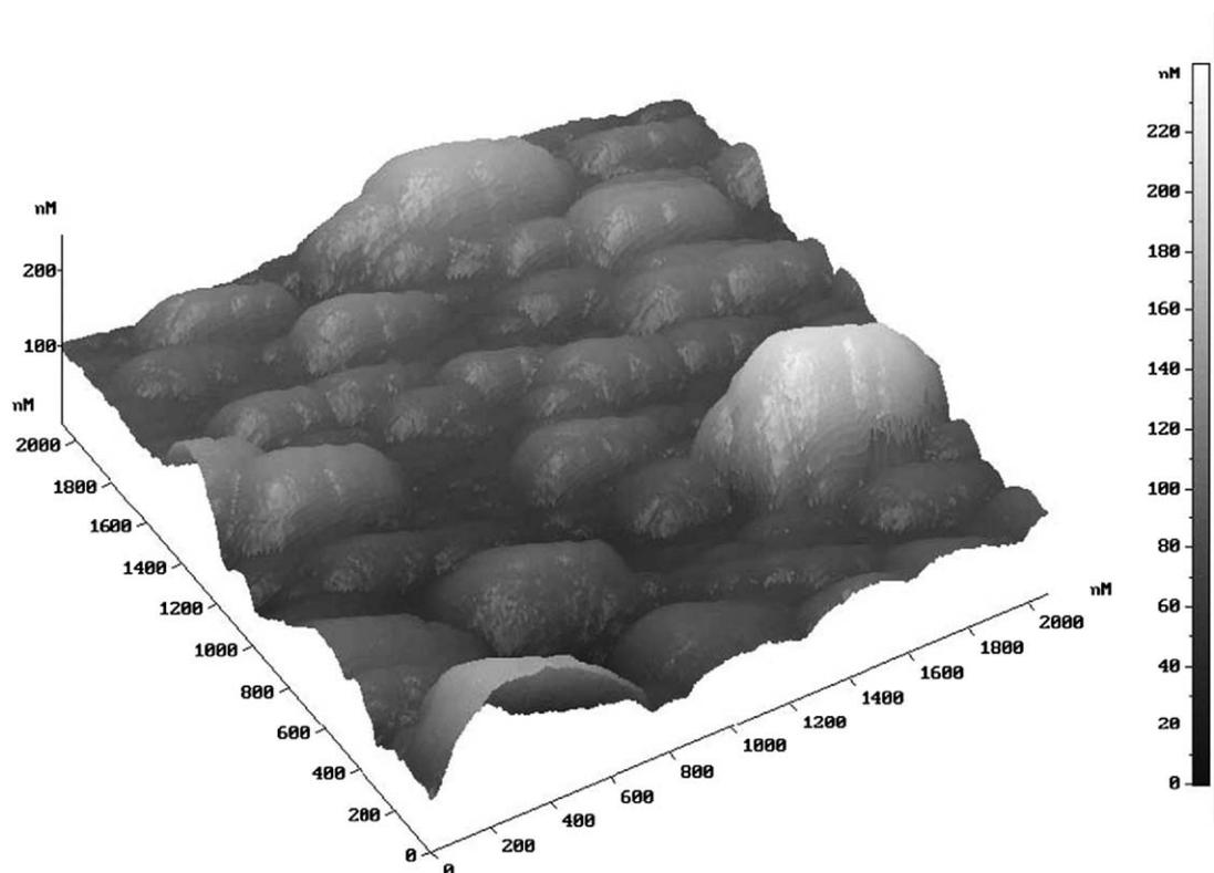
Fig. 2. AFM image of a typical surface morphology of SWNT/polymer films.
