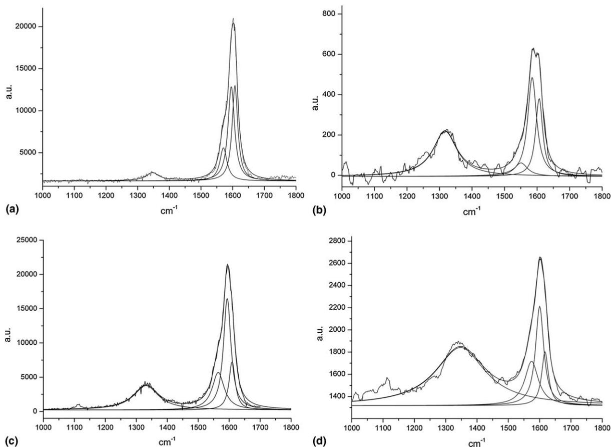
Fig. 5. Raman spectra in the region of the tangential modes of graphite taken from different samples of nanotubes: (a) untreated SWNT; (b) SWNT treated by KOH; (c) SWNT treated by HNO<sub>3</sub>; (d) SWNT treated by the HNO<sub>3</sub>/H<sub>2</sub>SO<sub>4</sub> mixture. The spectral data have been derived by curve fitting of the spectra to Lorentzian lines after background subtraction.
