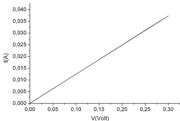
Fig. 7.  $I/V$  curve of a poly(1,8-DAN)/SWNT film ( $\text{HNO}_3/\text{H}_2\text{SO}_4$  treated nanotubes).
