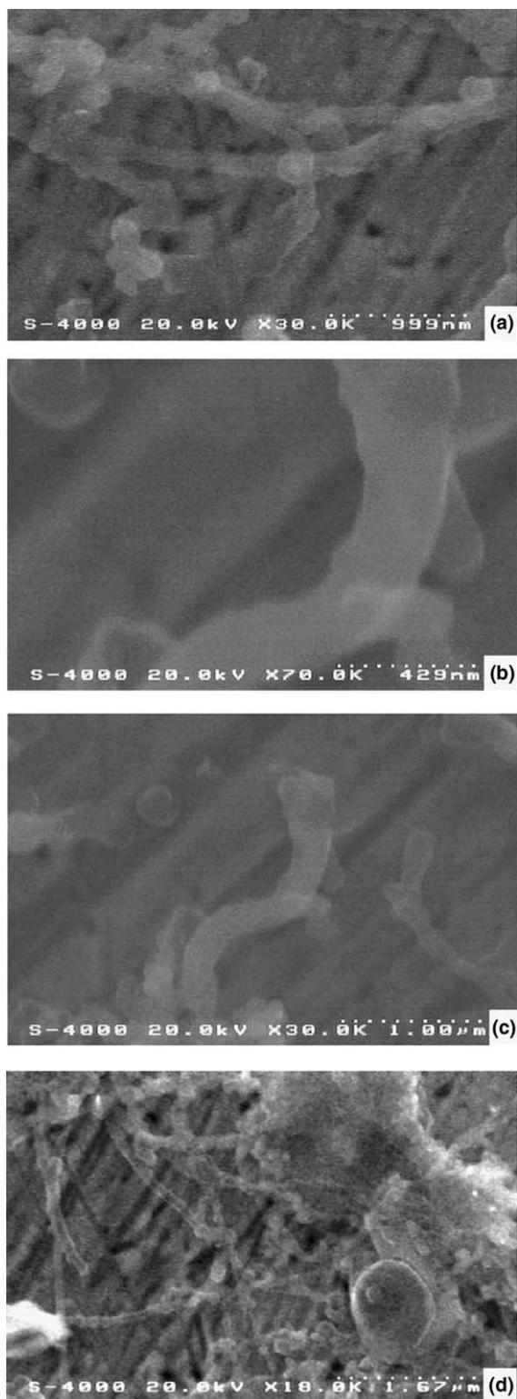
Fig. 3. FE-SEM images taken from a composite SWNT/polymer film after slight scratching of the top surface and showing: (a) shape and distribution of SWNT bundles and typical scratches of the Pt substrate; (b,c) details of SWNT bundles coated with polymer; (d) polymer aggregation in globular micro-islands.
