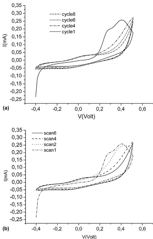
Fig. 1. Cyclic voltammograms for polymerization of 1,8-DAN at platinum electrode (sweep rate of 50 mV/s) from 0.1 M HClO<sub>4</sub> solution containing: (a) 1 mM 1,8-DAN; (b) 1 mM 1,8-DAN and 10 mg of SWNTs.
