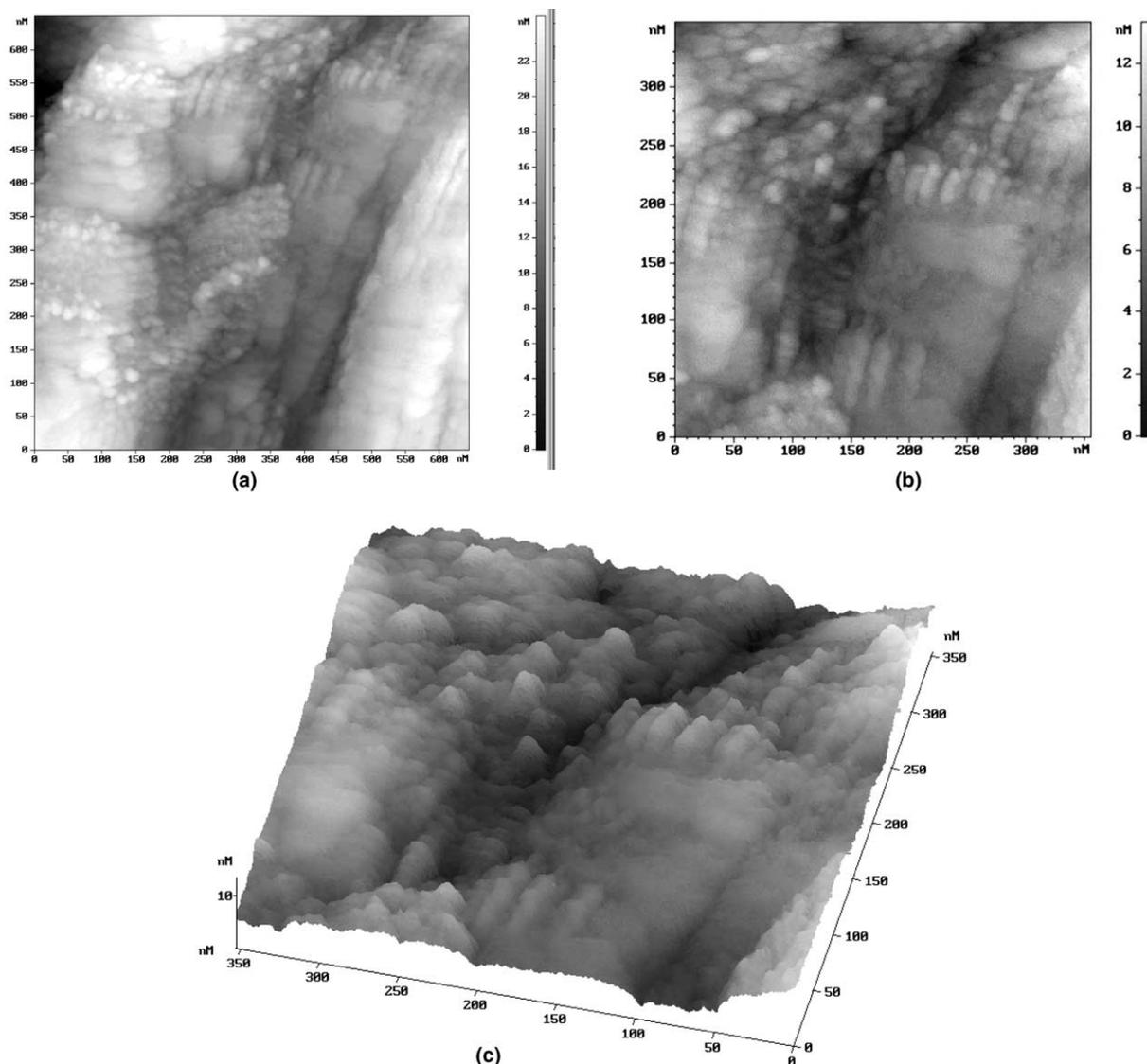
Fig. 4. Imaging by STM of SWNT bundles embedded in the polymeric matrix: (a) large scale image of an array of bundles contacting polymer micro-islands; (b) higher resolution of the same area; (c) top view micrograph showing the material microstructure on a 3-dimensional scale.
