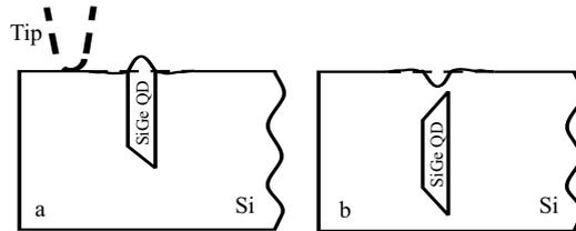
Figure 2: Illustration of elevation and depression appearance on the cleavage.
