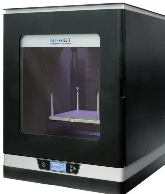
Figure 1. Photograph of the thermal cabinet.
