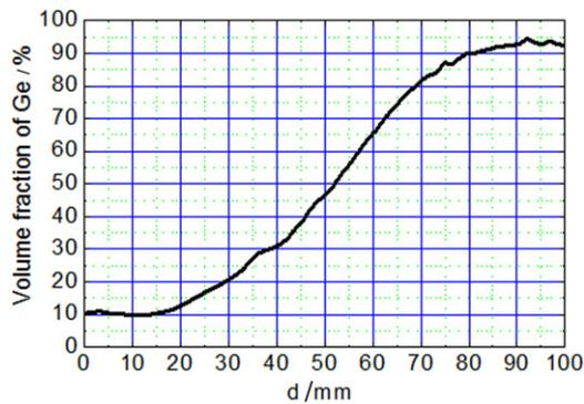
**Figure 1.** Fractional Ge phase content (given in vol%) as a function of the distance,  $d$ , from the low Ge content end of the film in the as-deposited (not annealed) Ge : SiO<sub>2</sub> layer (Ge-7).
