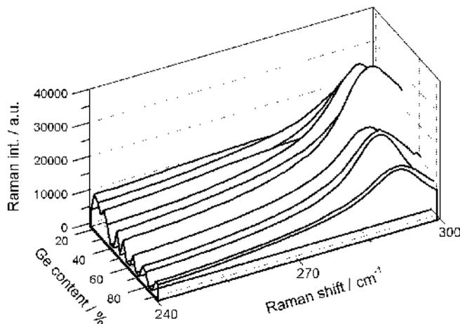
**Figure 4.** Raman spectra of the irradiated and annealed film, Ge-6, as a function of the Ge content along this film.
