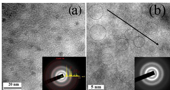
**Figure 3.** High-resolution TEM micrographs of the Ge : SiO<sub>2</sub> films with a Ge content of 83 vol% as obtained on the non-irradiated sample Ge-1 (a) and on the irradiated sample Ge-6 (b). The insets present the selected area diffraction (SAD) patterns of the corresponding layers. The SAD pattern in (a) also shows simulated ring patterns for amorphous Ge while the SAD pattern given in (b) clearly demonstrates the presence of Ge-NCs in the irradiated film.
