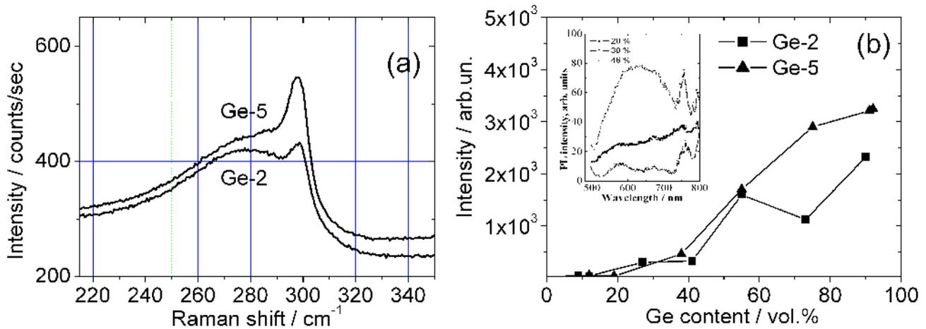
**Figure 6.** (a) Raman spectra as measured on the films with a Ge content of 75%. This is for the non-irradiated Ge-2 and the irradiated Ge-5 samples. (b) Ge content dependence of the integrated intensity of the NC peak in the Raman spectra. The inset shows the PL spectra for the irradiated sample Ge-5.
