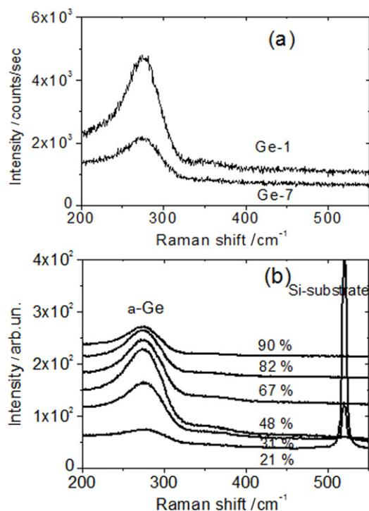
**Figure 2.** (a) Observed Raman spectra at  $d = 60$  nm (65% of Ge) for both, as-deposited sample Ge-7 and sample Ge-1, after the initial annealing. (b) Raman spectra of Ge-1 after additional annealing (500 °C for 20 min). The Ge contents at the measured positions along the film are indicated near the corresponding Raman traces. The Raman spectra are shifted along the vertical axis for convenience.
