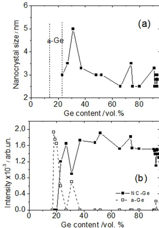
**Figure 5.** Size of the NCs (a) and the integrated intensity of the NC peak (b) as obtained from the Raman spectra dependence on the distance along sample Ge-6. The NC size was estimated from the position of the maxima of the NC peak in the Raman spectra while the integrated intensity of the spectra reflects the concentration of the NCs. Also shown is the relative intensity of the  $\alpha$ -Ge phase in the film.
