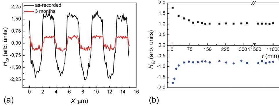
FIG. 3. (Color online) (a) Scanlines of the images shown in Fig. 1; 5 mins (black) and three months (red) after recording the grating. (b) Temporal decay of the grating: upper and lower curves present the relaxation of the positive and negative, i.e., bright and dark domain stripes in Fig. 1.
