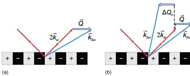
FIG. 6. (Color online) The scheme of the wave-vector (photon momentum) conservation for the cases of presence (a) and absence (b) of quasi-phase matching conditions for non-normal incidence.
