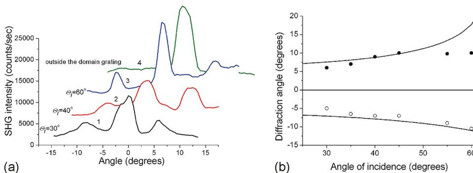
FIG. 5. (Color online) (a) The angular dependencies of the SHG intensity for different angles of incidence; the curve 4 is obtained when the fundamental beam is incident onto the crystal outside of the domain grating. (b) The diffraction angles of the “right” and “left” peaks as a function of the angle of incidence; the solid curves present fits using Eq. (2).
