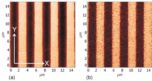
FIG. 1. (Color online) PFM images of an AFM-written domain grating 5 mins (a) and three months (b) after recording. The grating period is  $\Lambda = 3.6 \mu\text{m}$ . (The light and dark areas represent “positive” and “negative” domain stripes).
