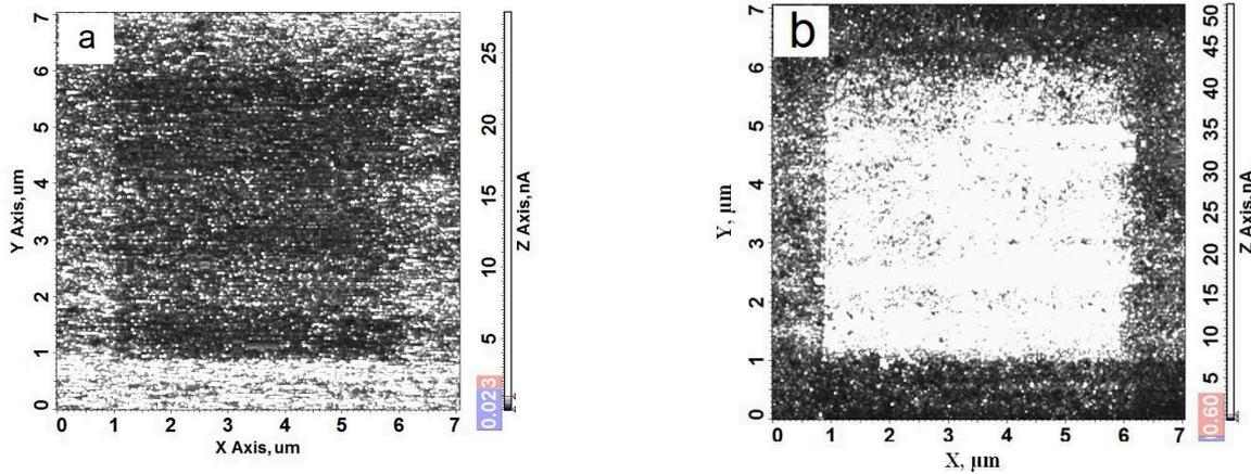
Fig. 1. AFM images of the current distribution on the surface of the silicon substrate, BDS-10 mark, obtained: a) - in air, b) - in an ultrahigh vacuum ( $10^{-8}$  Pa)
