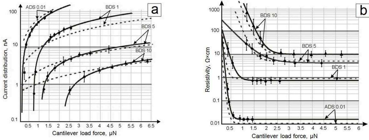
Fig. 2. The dependence of the electrical parameters of the silicon test samples from cantilever load forces between the probe tip to the sample surface: a) - the dependence of the current distribution; b) - the dependence of the resistivity. The dotted line - the theoretical dependence (1-7), the solid line –experimental dependence
