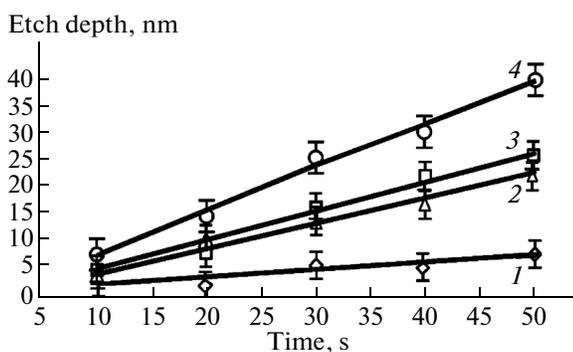
**Fig. 4.** Dependence of the etch depth of silicon on the exposure time for ion-beam currents: (1) 2.3, (2) 7.9, (3) 33.6, and (4) 111.4 pA.
