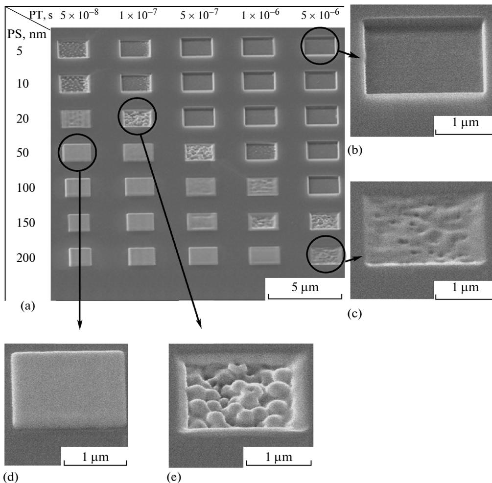
**Fig. 2.** SEM images of test-structure arrays obtained by the ion-stimulated deposition of Pt at an ion beam current of 7.9 pA.
