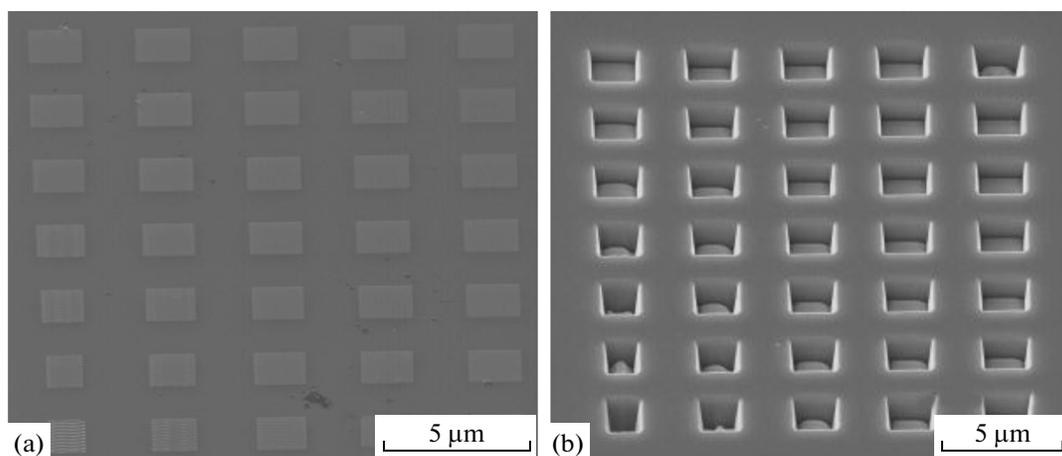
Fig. 1. SEM images of Pt structures arrays formed at (a)  $I = 2.3$  pA and (b)  $I = 511.4$  pA.
