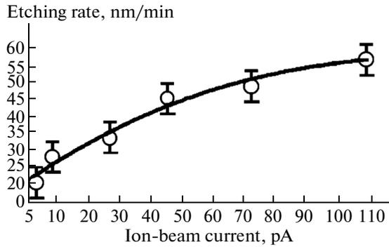
**Fig. 5.** Dependence of the rate of ion-beam etching of silicon on an ion-beam current.
