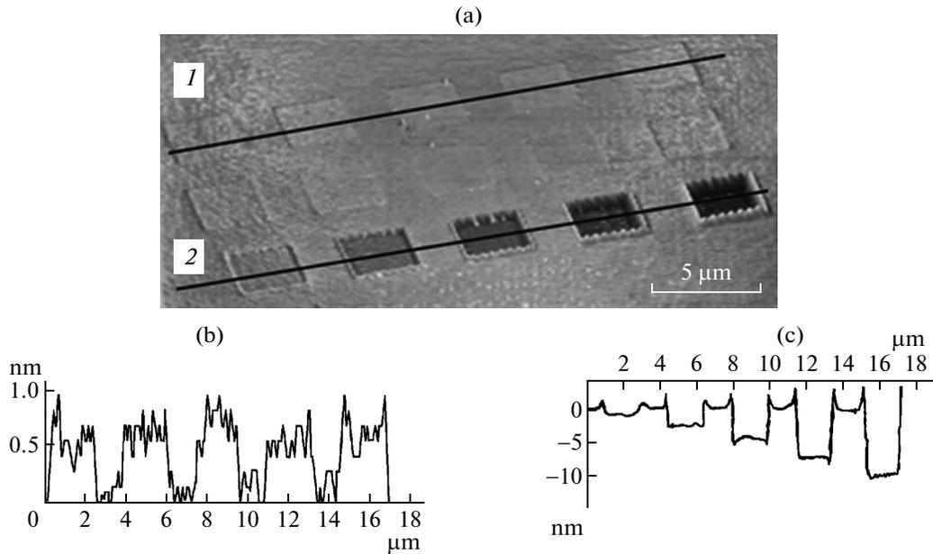
**Fig. 3.** Array of test structures obtained by ion-beam etching for  $I = 2.3$  pA: (a) AFM image, (b) profilogram along the line 1, and (c) profilogram along line 2.
