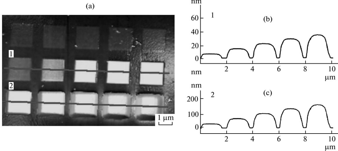
**Fig. 6.** An array of test structures obtained by the ion-stimulated deposition of Pt at  $I = 7.9$  pA: (a) AFM image; (b) profilograms.
