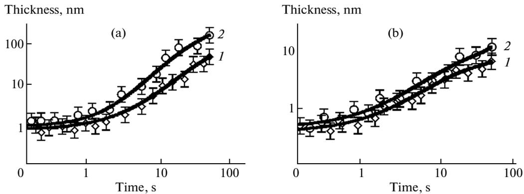
**Fig. 7.** Dependences of the thickness of the deposited layer on the ion-beam exposure time: (a) Pt and (b) W; (1)  $ST = 10$  ms; (2)  $ST = 50$  ms.
