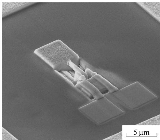
**Fig. 8.** SEM image of a prototype of a sensing element of the sensor accelerometer obtained on the basis of using the FIB method.
