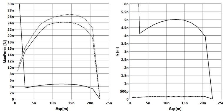
**Figure 2.** The plots of maximal tip-force (left) and sample depression (right) calculated with the Hertz model at different  $A_{sp}$  and for the samples with 100 MPa elastic modulus (solid line), with 2 GPa elastic modulus (dashed line) and with 70 GPa elastic modulus (dotted line).
