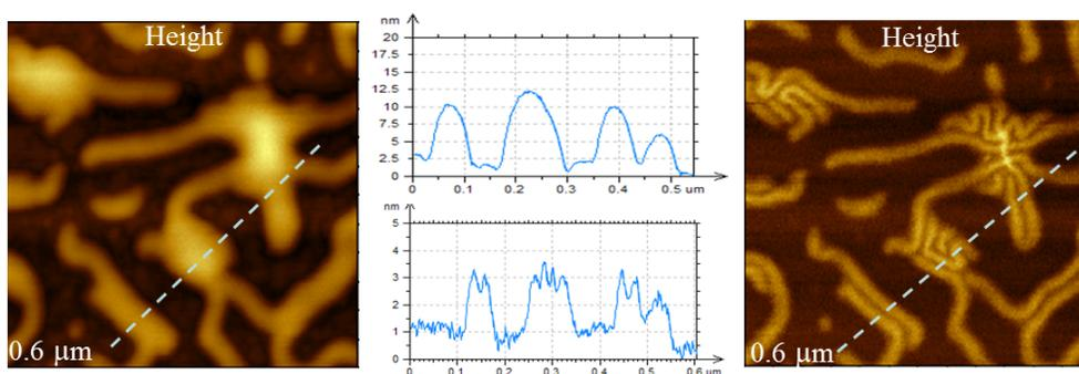
**Figure 3.** Height images and cross-sections of polymer brush macromolecules obtained in AC (left) and the non-resonant mode (right).
