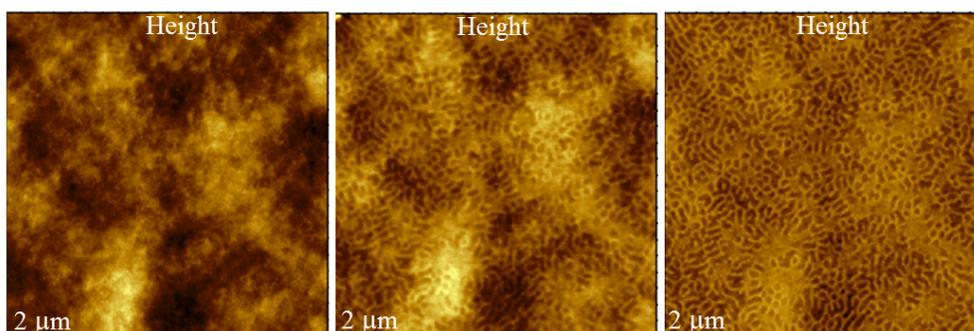
**Figure 4.** Height images of SBS triblock copolymer film obtained in AC (left, center) and the non-resonant mode (right).
