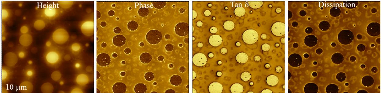
**Figure 5.** Images of PS/PB blend with the components' separation in contrast of various origin.
