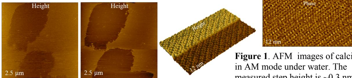
**Figure 1.** AFM images of calcite in AM mode under water. The measured step height is  $\sim 0.3$  nm
