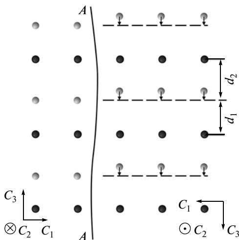
**Fig. 4.** Double layers of the bismuth crystal in blocks of two orientations with the opposite direction of the crystallographic axes. The  $A-A$  line is the boundary between the blocks. Short arrows indicate the atomic displacement during annealing of the film,  $d_1 = 0.160$  nm is the distance between the atomic planes inside the double layer, and  $d_2 = 0.236$  nm is the distance between the nearest atomic planes of the neighboring double layers.
