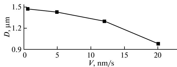
Fig. 1. Influence of the deposition rate on the average size of the crystallites. The film thickness is 300 nm.  $T_{\text{sub}} = 110^\circ\text{C}$ . The films are unannealed.
