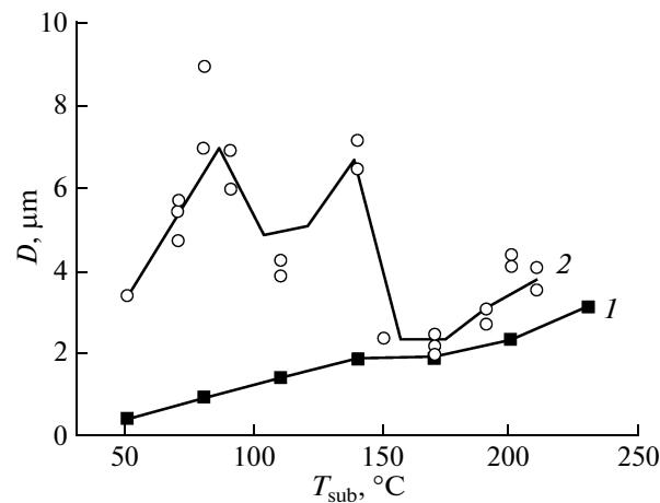
Fig. 2. Influence of the temperature of the substrate and annealing on the average size of the crystallites (1) before and (2) after annealing. The film thickness is 300 nm.
