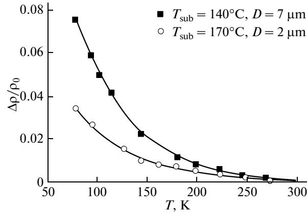
Fig. 3. Influence of the crystallite size in films 300 nm thick on the magnetoresistance.
