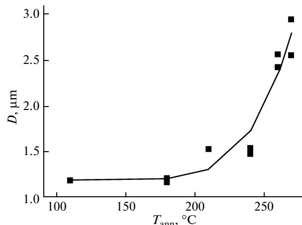
Fig. 5. Dependence of the average crystallite size on the annealing temperature. The initial films 100 nm thick were prepared at a substrate temperature of 110°C. The annealing time for all films was 30 min.
