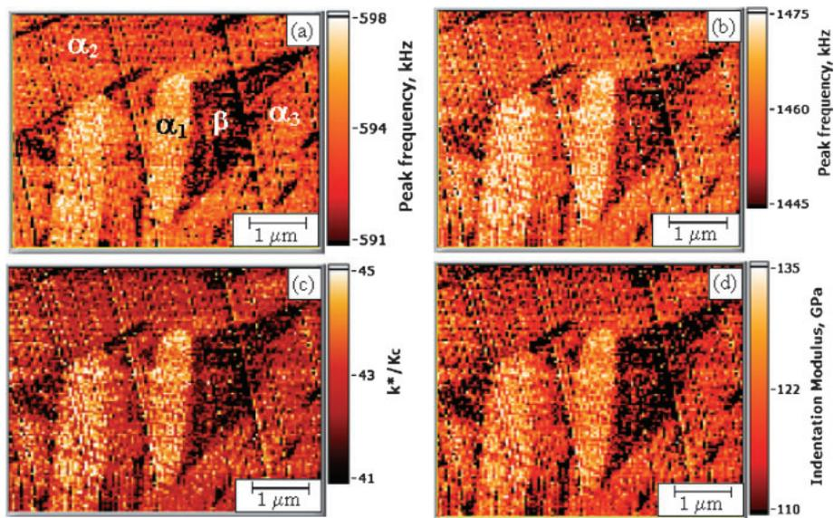
Fig. 2. (a) Distribution of first contact-resonance frequency, (b) second contact-resonance frequency, (c)  $k^*/K_c$ , and (d) indentation modulus of the Ti-6Al-4V specimen heat treated at 1123 K for 1 h followed by water quenching. The three different variants of alpha phase are marked in (a) as  $\alpha_1$ ,  $\alpha_2$ , and  $\alpha_3$  in decreasing order of their indentation modulus as observed experimentally.
