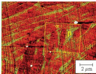
Fig. 1. Tapping mode topographic image of the Ti-6Al-4V sample showing the area selected for the AFAM measurements ( $z$ -scale = 4 nm).
