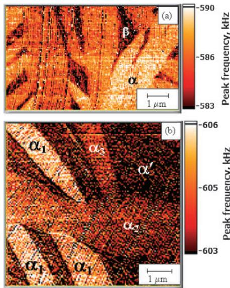
Fig. 3. Distribution of the first contact-resonance frequency in the Ti-6Al-4V specimens heat treated at (a) 1123 and (b) 1223 K for 1 h followed by water quenching. The three different variants of alpha phase are marked in (b) as  $\alpha_1$ ,  $\alpha_2$ , and  $\alpha_3$  in decreasing order of their indentation modulus as observed experimentally.
