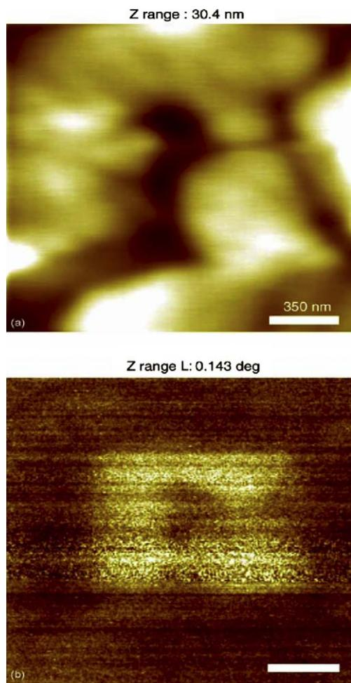
Fig. 5. Piezoresponse AFM images of polarization patterned PZT film: (a) topography, (b) phase of the piezoresponse signal. Non-piezoelectric pyrochlore region is visible in the center of patterned area. Bar = 0.35  $\mu\text{m}$ .
