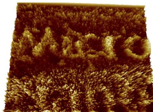
Fig. 6. Polarization-patterned PZT film with complex patterns in the form of written words “micro, nano” ( scan area:  $1 \times 1 \mu\text{m}^2$ ).
