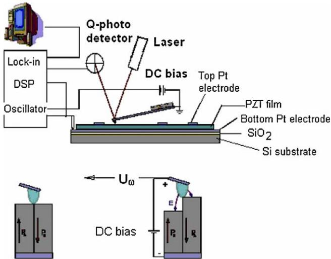
Fig. 1. AFM based experimental setup to measure local piezoresponse.
