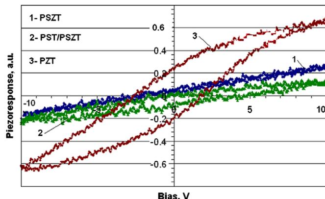
Fig. 4. Piezoresponse AFM hysteresis loops: (1)–unpoled; (2)poled.
