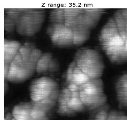
Fig. 2. AFM image of surface microstructure of the PZT film ( scan area:  $1 \times 1 \mu\text{m}^2$ ).
