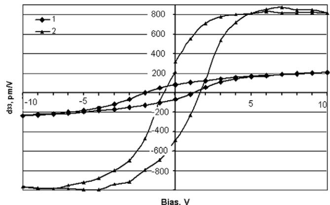
Fig. 3. Piezoelectric coefficient  $d_{33}$  hysteresis loops of PZT film measured by Doppler vibrometer: (1)–unpoled; (2)–poled.
