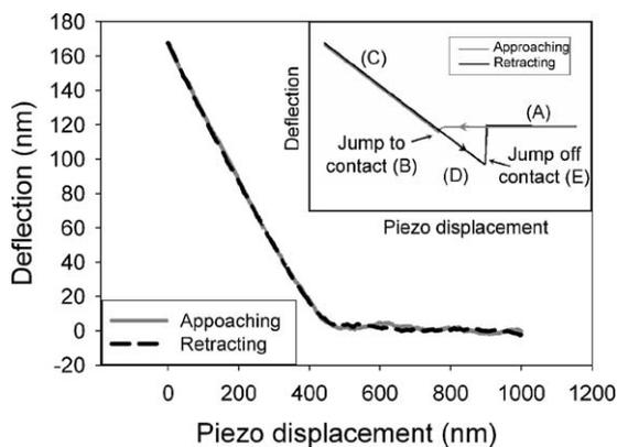
Fig. 3. Typical deflection vs. piezo displacement curve obtained on a coated yeast cell in liquid ( $[\text{NaCl}] = 0.5 \text{ M}$ ). Scan rate:  $0.5 \mu\text{m/s}$ . Inset: generic deflection vs. piezo displacement curve (see Appendix A for a description).
