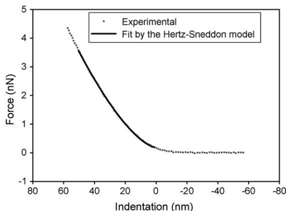
Fig. 6. Typical force vs. indentation curve of a coated yeast cell: experimental data (dotted line) and data generated using the Hertz–Sneddon model (solid line).
