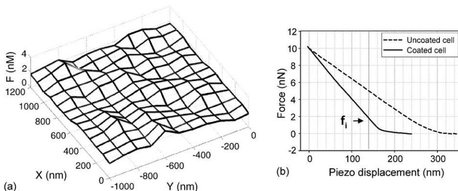
Fig. 5. (a) Force map obtained on a  $1.2 \mu\text{m} \times 1 \mu\text{m}$  region of a coated yeast cell by plotting the  $f_i$  values calculated by cutting the force curves, previously superimposed at a chosen force value (10 nN in this case), at a chosen piezo displacement (140 nm in this case) as shown in (b). According to this analysis stiffer samples are characterized by lower  $f_i$  values.
