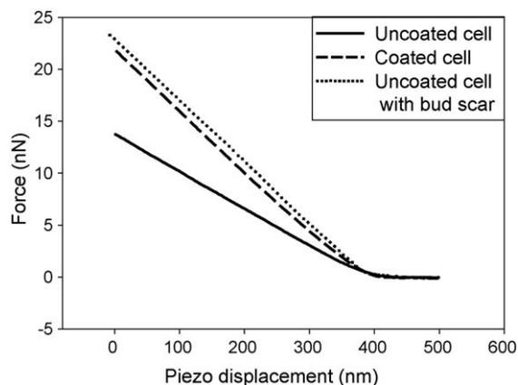
Fig. 4. Typical force vs. piezo displacement approaching curves for coated cells (dashed line), uncoated cells (solid line) and uncoated cells in the bud scar region (dotted line).
