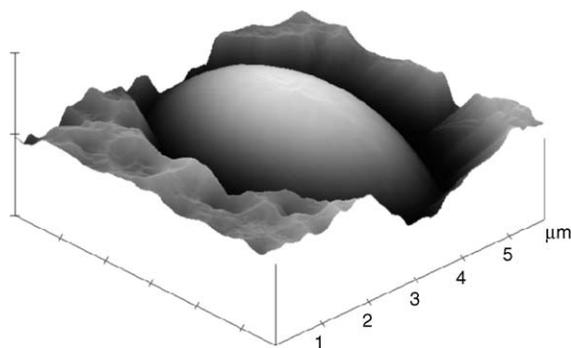
Fig. 1. 3D rendered AFM height image of an encapsulated cell trapped in a pore of a polycarbonate membrane in liquid ([NaCl] = 0.5 M); image size: 5.7  $\mu\text{m} \times 5.7 \mu\text{m}$ ; z scale: 1  $\mu\text{m}/\text{div}$ .
