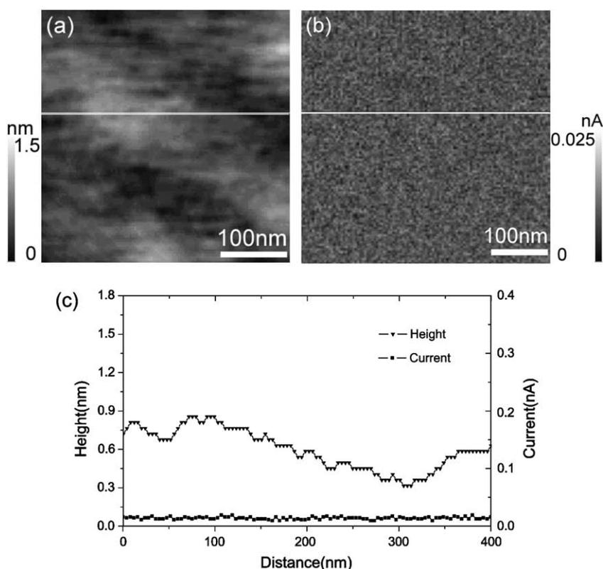
Fig. 3. Topographic (a) and current (b) images of Ge QDs grown at 550 °C after etching in 30%  $H_2O_2$  solution for 30 min. Both images were obtained simultaneously at a sample bias voltage of 1.0 V and the scan size was 400 nm  $\times$  400 nm. (c) Respective cross-sectional profiles along the solid lines marked in (a) and (b).
