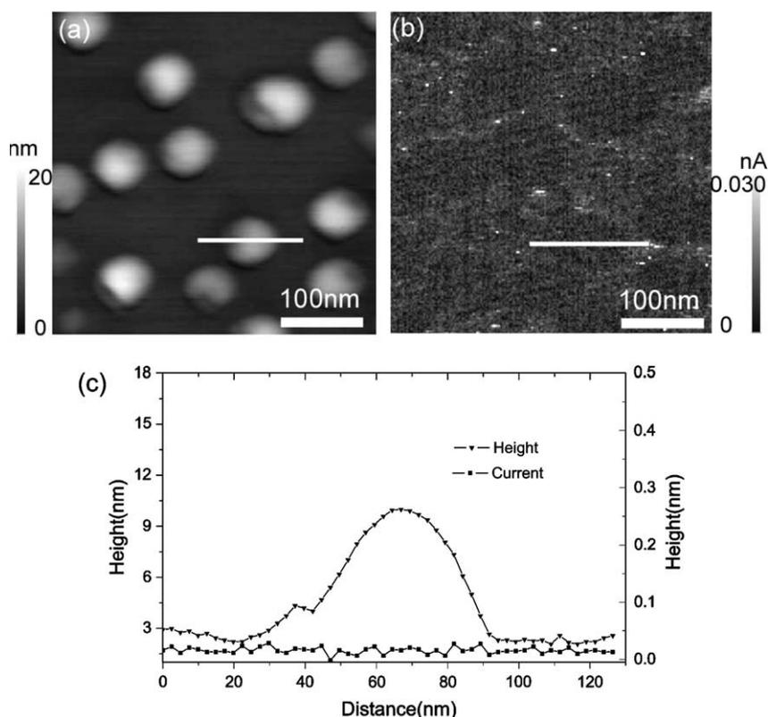
Fig. 4. Topographic (a) and current (b) images of Ge QDs grown at 640 °C after etching in 30%  $\text{H}_2\text{O}_2$  solution for 30 min. Both images were obtained simultaneously at a sample bias voltage of 1.9 V and the scan size was  $400 \text{ nm} \times 400 \text{ nm}$ . (c) Respective cross-sectional profiles along the solid lines marked in (a) and (b).
