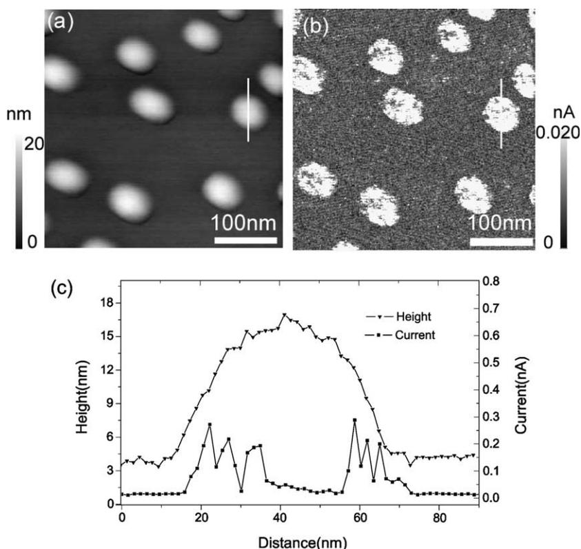
Fig. 2. Topographic (a) and current (b) images of Ge QDs grown at 640 °C. Both images were obtained simultaneously at a sample bias voltage of 1.4 V and the scan size was 400 nm × 400 nm. (c) Respective cross-sectional profiles along the solid lines marked in (a) and (b).
