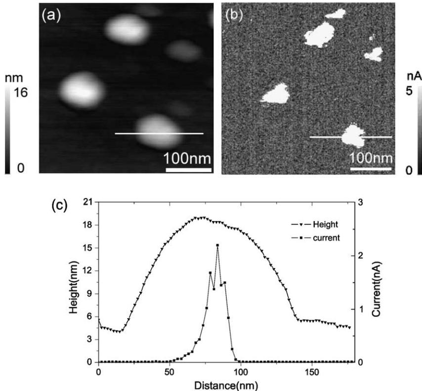
Fig. 1. Topographic (a) and current (b) images of Ge QDs grown at 550 °C. Both images were obtained simultaneously at a sample bias voltage of 1.0 V and the scan size was 400 nm  $\times$  400 nm. (c) Respective cross-sectional profiles along the solid lines marked in (a) and (b).
