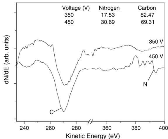
Fig. 8. AES spectra of the 350 and 450 V samples.
