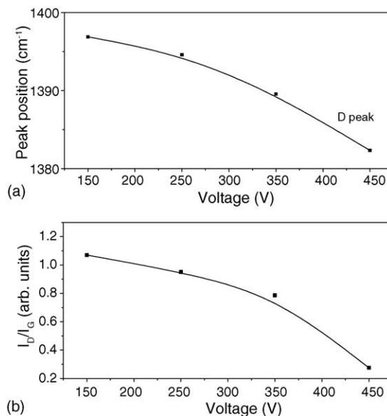
Fig. 5. The Dependence of (a) D peaks position (b)  $I_D/I_G$  with respect to voltage from the IR spectrum.
