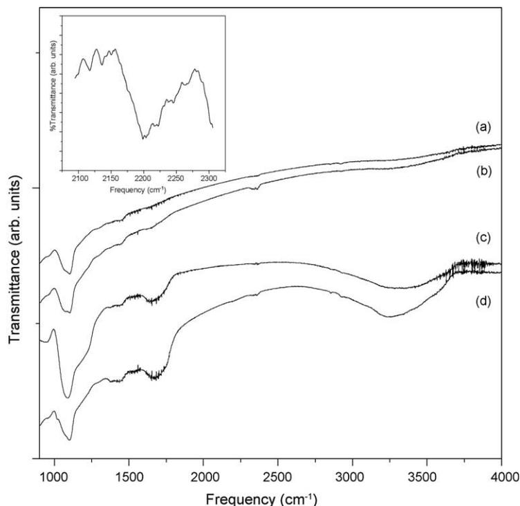
Fig. 3. Typical IR transmission spectrum of the samples: (a) 150 V (b) 250 V (c) 350 V (d) 450 V.
