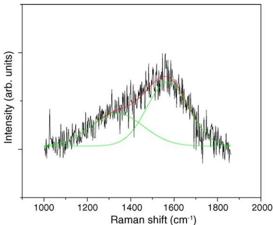
Fig. 6. Typical deconvolution of the Raman spectra of one of the samples.
