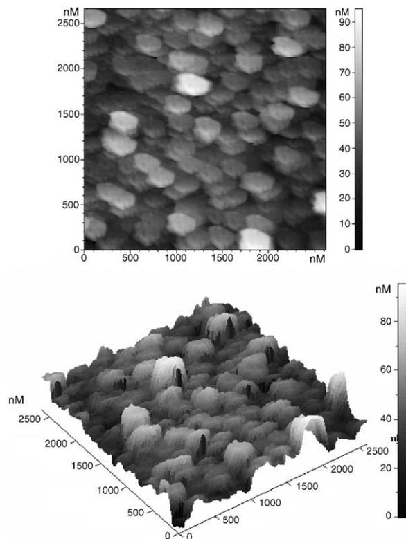
Fig. 2. AFM pattern of the sample prepared at 250 V.
