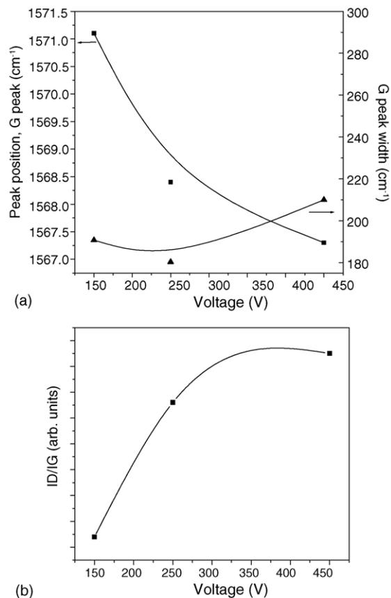
Fig. 7. The Raman spectrum of the films: (a) right Y-axis (filled triangles) G peak width, left Y-axis (filled squares) G peak position and (b)  $I_D/I_G$  with respect to voltage.
