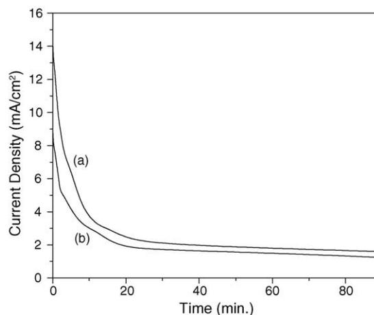
Fig. 1. The current density–time behavior of the samples deposited at (a) 250 V (b) 150 V.
