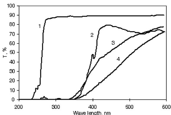
Fig. 3. Transmission spectra for PMMA samples in UV- and visual ranges: without an addition agent 0 Mrad (1); PMMA containing fullerene  $C_{60}$  ( $9 \times 10^{-3}$  mol/kg) 0 Mrad (2), 10 Mrad (3), 30 Mrad (4).
