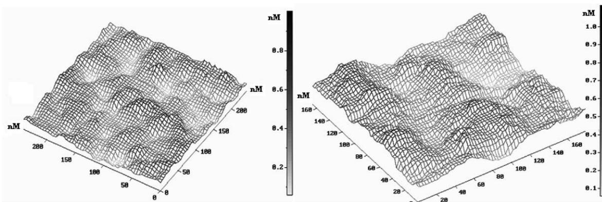
Fig. 4. Topography of PMMA films surface with fullerene presence and without it.
