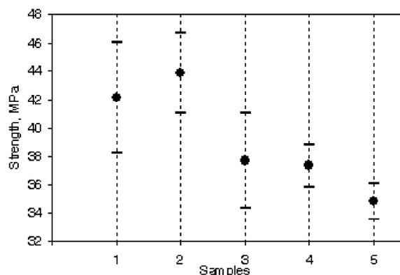
Fig. 2. Rupture strength of the examined PMMA films containing no addition agent 0 Mrad (1), 10 Mrad (5); PMMA containing  $C_{60}$  ( $8.5 \times 10^{-3}$  mol/kg) 0 Mrad (2), 5 Mrad (3), 10 Mrad (4).
