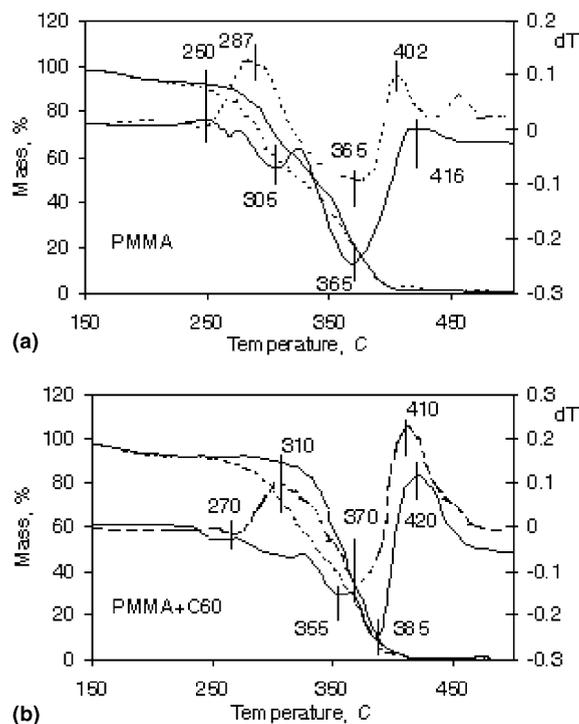
Fig. 1. Results of the investigations for thermoxidative destruction of PMMA films in the air medium: *solid line*—nonirradiated samples; *dotted line*—samples after their radiation treatment with dose 10 Mrad; *numerical designation*—typical value of temperature.
