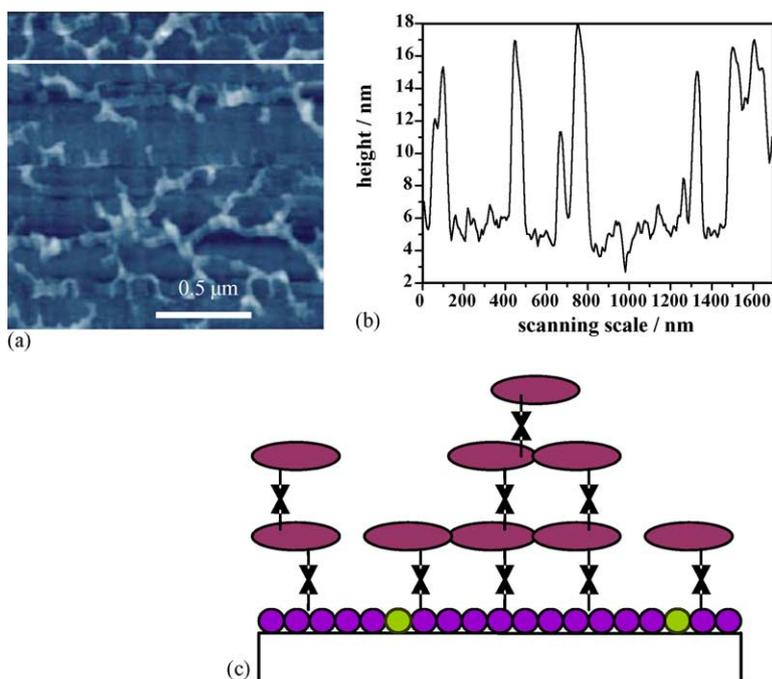
Fig. 6. Protein adsorption on the mixture 1:10: (a) topography of protein pattern on the mixture 1:10, (b) cross section of the line in (a), (c) schematic illustration for the protein adsorption on the mixture 1:10 SAMs.
