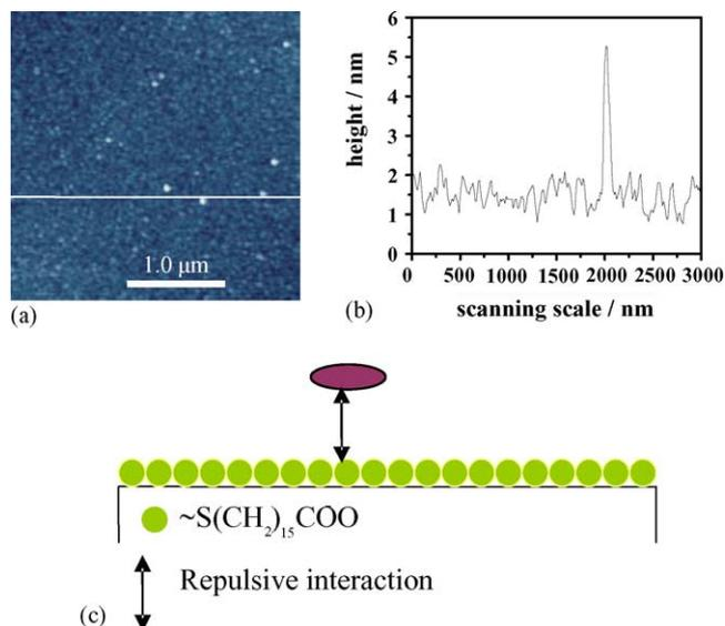
Fig. 3. Protein adsorption on MHA SAMs: (a) topography of protein pattern on MHA SAMs, (b) cross section of the line in (a), (c) schematic illustration for the adsorption MHA SAMs.
