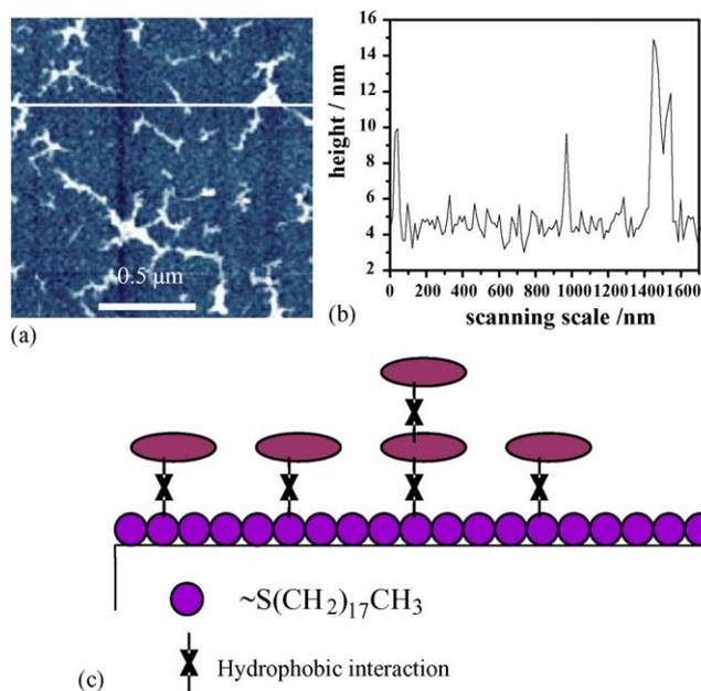
Fig. 4. Protein adsorption on ODT SAMs: (a) topography of protein pattern on ODT SAMs, (b) cross section of the line in (a), (c) schematic illustration for the protein adsorption on ODT SAMs.
