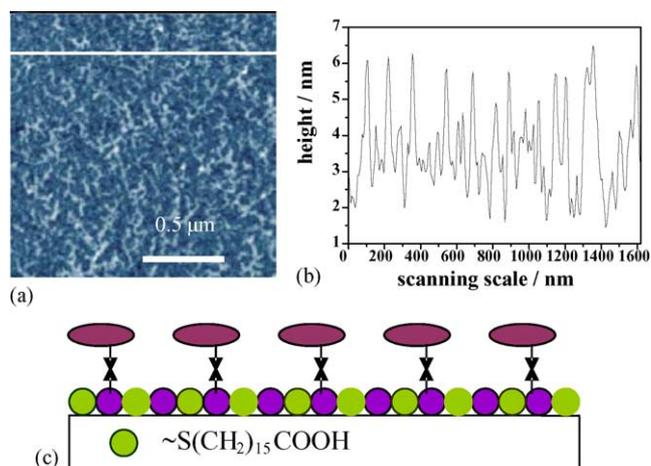
Fig. 5. Protein adsorption on the mixture 1:1 SAMs: (a) topography of protein pattern on the mixture 1:1 SAMs, (b) cross section of the line in (a), (c) schematic illustration for the protein adsorption on the mixture 1:1 SAMs.
