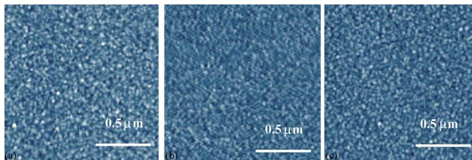
Fig. 1. Topography of gold film and SAMs: (a) topography of gold film, (b) topography of ODT SAMs, (c) topography of the mixture 1:1 SAMs.
