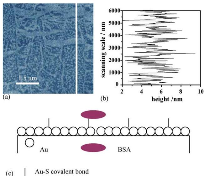
Fig. 2. Protein immobilization on gold film: (a) topography of gold after adsorb BSA, (b) cross section of the line in (a), (c) schematic illustration for the protein immobilization on gold film.
