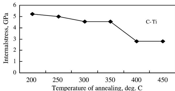
Fig. 5. Dependences of change of internal stress value on temperature of annealing in carbon condensates with general thickness  $1.0\ \mu\text{m}$  with interlayers of titanium with thickness  $200\ \text{nm}$ , obtained at the temperature of a sublayer  $100\ ^\circ\text{C}$ .
