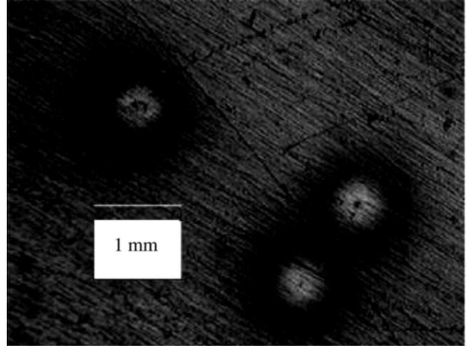
Fig. 3. Zones of change of coatings thickness caused by diffusion processes in places of defects.
