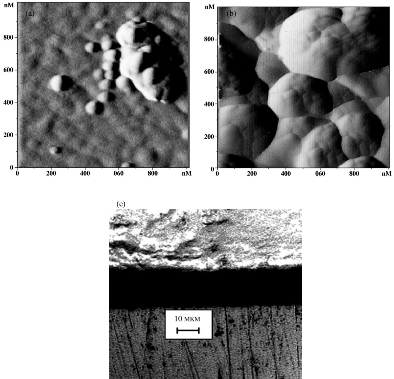
Fig. 1. Superficial structures of a carbon condensate with thickness 300 nm (a) and 10  $\mu\text{m}$  (b); (c) an appearance of a superhard carbon coating with thickness 10  $\mu\text{m}$  on a sublayer from silicon after cross microgrinding.
