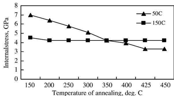
Fig. 4. Dependences of change of internal stress value on temperature of annealing in carbon condensates obtained at the temperature of a sublayer 50, 100 and 150°C and duration of a pulse of discharge 0.7 ms.
