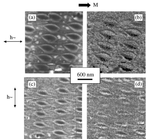
Fig. 2. AFM topography (a,c) and the corresponding images of the dynamic response (b,d). The dynamic images have been collected at different orientations of the AC field,  $\vec{h}_{\sim}$ , with respect to the entities' magnetization,  $\vec{M}$ : (b)  $\vec{h}_{\sim} \parallel \vec{M}$ , (d)  $\vec{h}_{\sim} \perp \vec{M}$ . Unlike MFM, these images indicate that the patterned ferromagnetic entities have a ring shape.
