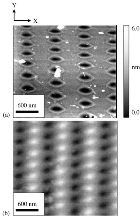
Fig. 1. AFM (a) and MFM (b) images of the patterned entities in a 15-nm thickness Fe–Cr film. The MFM image indicates the formation of single-domain ferromagnetic entities in the interference maxima. However, the magnetic features of the entities are not clear in detail.
