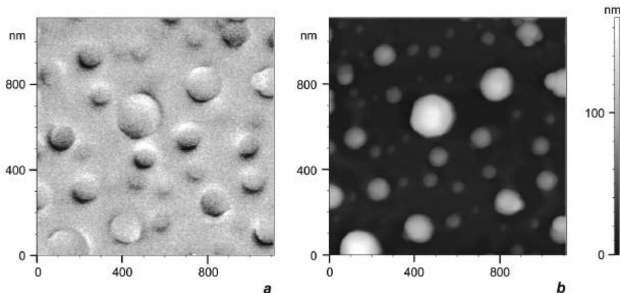
**Figure 3.** MFM image (a) and the topography (b) of an area of a sample with separate nickel nanoparticles formed on the silicon dioxide surface.
