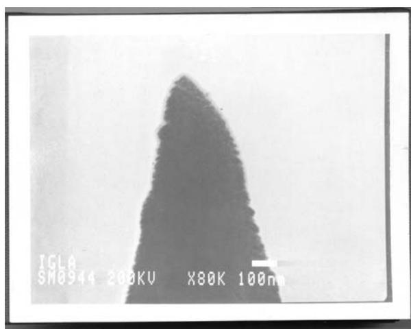
Fig. 1. Probe for surface modification on the base of optical fiber
