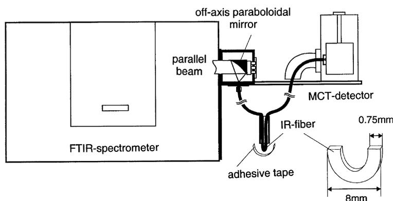
Fig. 1. Experimental set-up with a FTIR-spectrometer and the silver halide fiber-optic probe.
