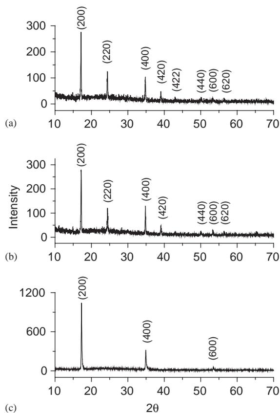
Fig. 1. XRD patterns of: (a)  $\text{Co}_3[\text{Fe}(\text{CN})_6]_2 \cdot n\text{H}_2\text{O}$  precipitate formed without ODA monolayer; (b) Co-hcf precipitate formed at the bottom of the trough in presence of ODA monolayer; and (c) Co-hcf film formed at the air–water interface and transferred on glass.
