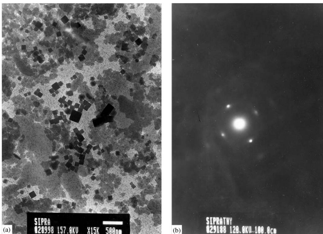
Fig. 2. Transmission electron micrograph (a), and the ED pattern (b) of Co-hcf film grown under ODA monolayer for 6 days and transferred on carbon coated copper grid.
