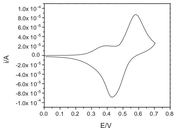
Fig. 4. Cyclic voltammogram of Co-hcf film (transferred gold-coated glass electrode) in 0.1M KCl solution. (Scan rate = 50 mV/s Reference Electrode is Ag/AgCl.)
