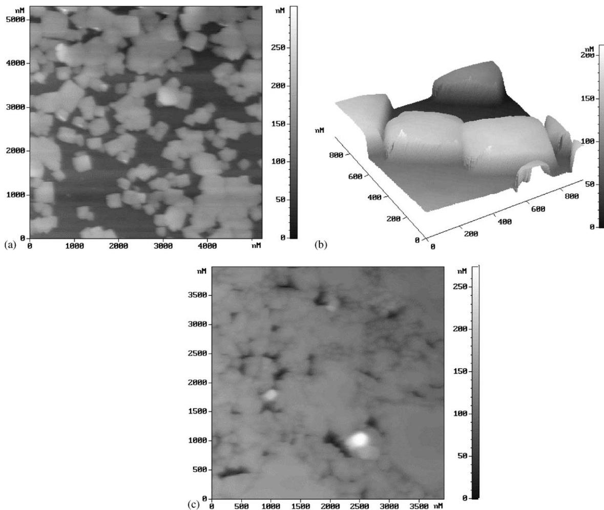
Fig. 3. AFM images of selected areas of Co-hcf film grown at air–water interface under the ODA monolayer and transferred on mica substrate. (a) two-dimensional image of area  $5000 \times 5000 \text{ nm}^2$ ; (b) three-dimensional image of area  $900 \times 900 \text{ nm}^2$ ; and (c) two-dimensional image of area  $4000 \times 4000 \text{ nm}^2$ . (a) and (b) pertain to a film grown over a period of three days whereas (c) depicts the film grown for six days.
